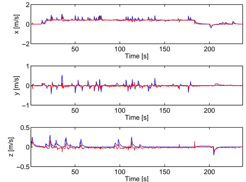
The linear velocities predicted using the hydrodynamic model are slightly overestimated. Some artifacts may possibly be explained by currents and turbulence not accounted for in the model, also there is noise in the DVL measurements.
